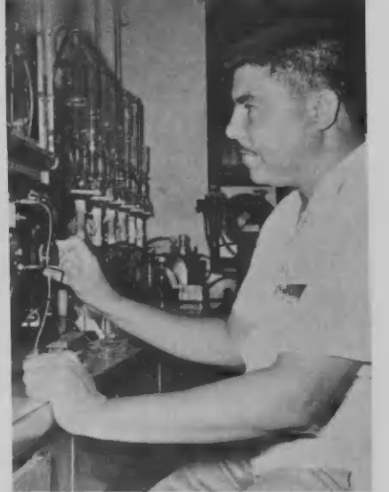
TEL CONTENT of gasoline is being determined on the Polarograph by Juan Ras. CONTENIDO DI chumbo den gasolin ta ser determiná pa J. Ras riba e Polarograph.
